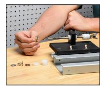
1. To install your thread carriage magnets, unscrew the wing nut, metal washers and tension spring. Leave one small bushing in place.
