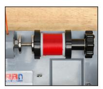
2. Install the **small washer** first then add the **two magnets**. Your magnets are marked P and N for their polarities, be sure their polarities are facing each other. Once the magnets are installed you will replace the **washers**, **spool retainers**, **thread spool and precision knob** in the same order you removed them.
