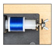
2. After sliding your desired thread spool into place, install the 2 bushings, 2 washers, then add the two magnets. Your magnets are marked P and N for their polarities, be sure their polarities are facing each other. Once the magnets are installed you will tighten the wing nut to set desired tension.
