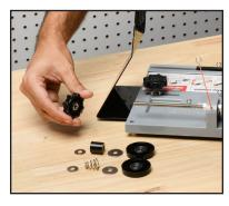
1. To install your thread carriage magnets, unscrew the **precision knobs** and remove all **washers**, **thread spool** and **tension spring** from the threaded rod.
