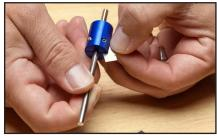
2. To attach blades, use the provided hex key to loosen each set screw. Slide the cutting blades into the blade slot and be sure they are properly seated. The notches in the blades should be facing out. The blades should be set straight in the blade slots. Once each blade is properly seated, tighten the set screw to secure each blade.
