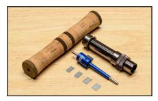
1. Once you unbox your inletting tool, measure the size of the inlet hole you wish to cut. If you are cutting a hole to fit a fly reel seat, measure the fly seat hood outside diameter and match that size to one of the 5 blade sizes. When working with cork be sure to cut a hole to match or slightly larger as cork does not stretch.
