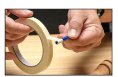
3. Once your blades are set, check to be sure your 6mm guide sleeve will properly fit the inner diameter of your grip or cork/EVA ring. If the inner diameter is larger than .250" you will need to arbor the 6mm guide sleeve to be sure of a straight and consistent cut. We recommend using masking tape to arbor the sleeve. Allow enough room for the sleeve to slide freely, as the inlet tool cuts into the grip.
